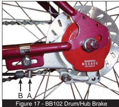
Figure 17 - BB102 Drum/Hub Brake
