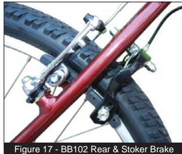
Figure 17 - BB102 Rear & Stoker Brake
